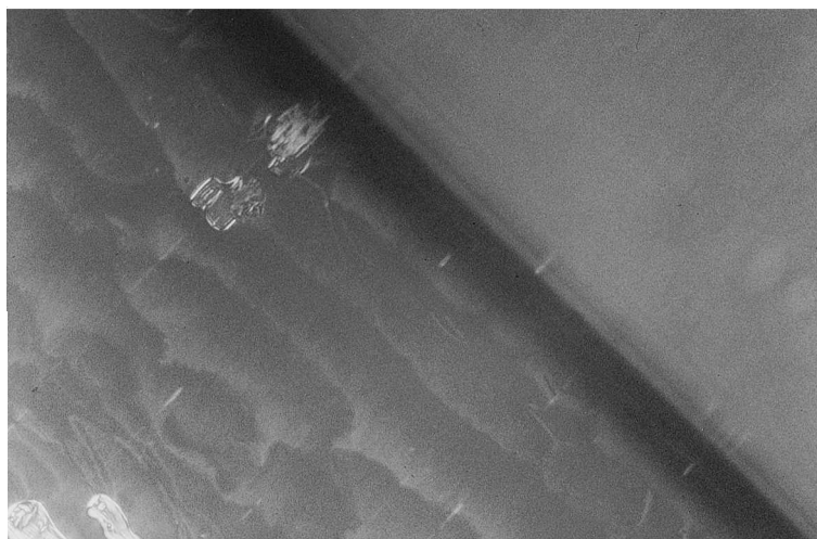
Figure 13. TGBA phase with Grandjean-Cano texture for n = 14 at 98^\circ\text{C} .
